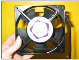
120mm computer fan fits 150mm ducting easily
